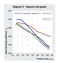
KSE 3.0: RATED DISCHARGE COEFFICIENTS  $\alpha_w$  AS FUNCTION OF h/d $_0$  AND  $p_{a0}/p_0$
