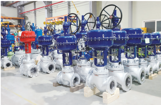
V100 Series and V200 Series, high-performance flanged globe control valves, ensure precise flow, pressure and temperature control, as well as reliability in critical chemical, petrochemical, and oil & gas plants within demanding industrial environments.
