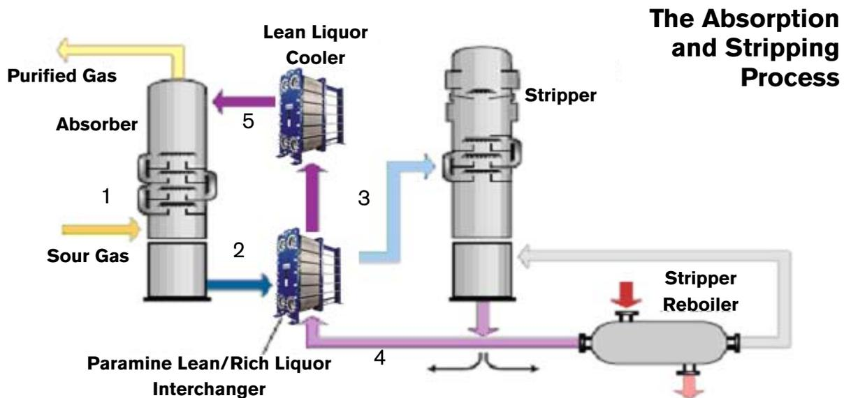
1. The sour gas streams enter the bottom of the Absorber column and flows upward counter-current to the lean liquor solution. The liquor picks up the gases in the solution and leaves the bottom of the column, due to the exothermic absorption reaction. The Purified Sweet Gas, after absorption, flows overhead from the Absorber.
