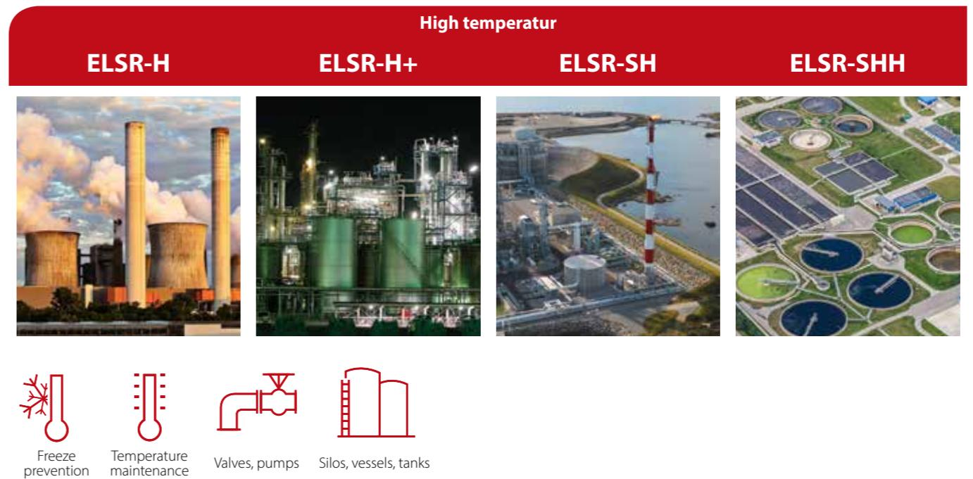
The ELSR-H, -H+, -SH and -SHH high temperature trace heater range is designed for temperature maintenance in industrial processes and applications in hazardous areas. The trace heaters' high chemical resistance allows them to be installed in environments with exposure to aggressive influences.
