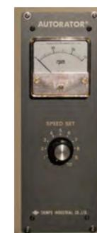
In addition to the standard handle operation, there is also an automatic control panel that can be controlled remotely to adjust the rotation speed.
